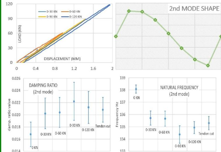
The vibration response is highly sensitive to the tendon cut and it can be used for damage detection.
